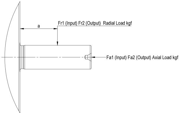
Gearbox Input Fa1 Fr1 at 1000 n<sup>-1</sup> Gearbox Output Fa2 Fr2 at 100 n<sup>-1</sup> a=distance from gearbox face to load center. \* = see product page for where a is from.
